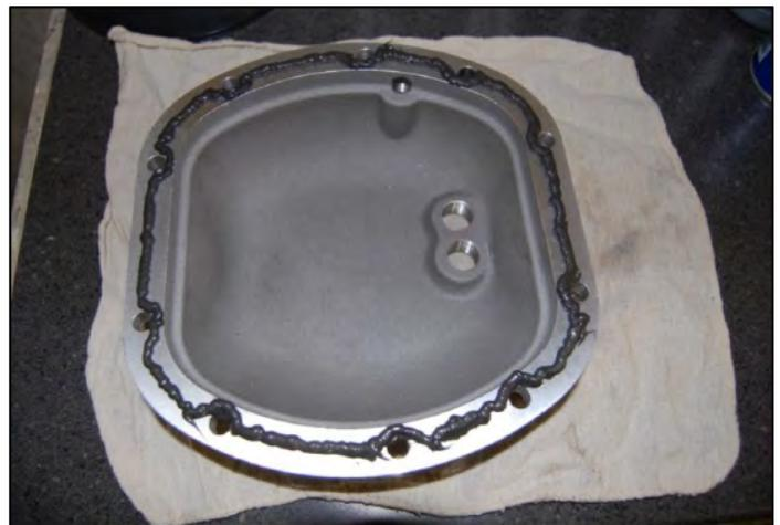
11. Install the rest of the supplied bolts and washers and torque to 15 ft/lb. in a crisscross pattern.
