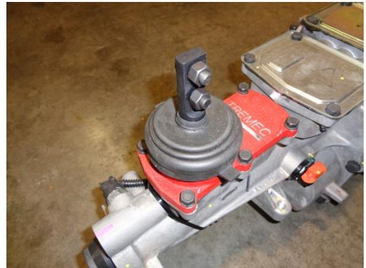
The shifter boot that is included with the stock Tremec shifter can be re-used on the Hurst shifter. To use this boot, it will need to be modified by cutting off the bottom section of the boot as shown.
