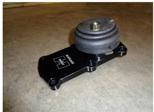
The shifter “body” will be in the rear position on the rear TKO shifter cavity. Make sure the pivot ball is positioned into the rear socket and that the white plastic bushing is still in place.
